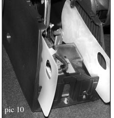
11. Installing the base attachment bracket is the most difficult step of the installation. While lifting the console and spreading the rear opening of the console, insert the base attachment bracket through the rear of the console. The plastic sheets will make the job much easier.
