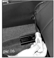
completely tighten at this stage. The rear screws will now secure the center console and the base attachment piece to the steel pillars with the red screw anchors we discussed in step 12. It is very important that both sides align correctly and the screws are reinstalled properly. (pic 15 &16)
