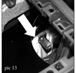
ment bracket must be pushed straight down over the pillars to insure the red screw anchors stay in place. See illustration. (pic 13)
