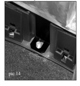
14. After the base attachment bracket is correctly in position in the center console and all three holes align properly, re-install the rear most #20 torx head screws into the sides of the center console. Do not
