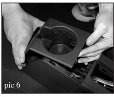
6. After the front edge of the cup holder insert is disengaged from center console, use a pry tool to remove the two nylon trim panel retainers from the bottom rear of the cup holder insert piece and remove the cup holder insert from center console. Put the two nylon trim panel retainers somewhere safe as you will reuse them. The cup holder insert will not be re-used. (pic 6)
